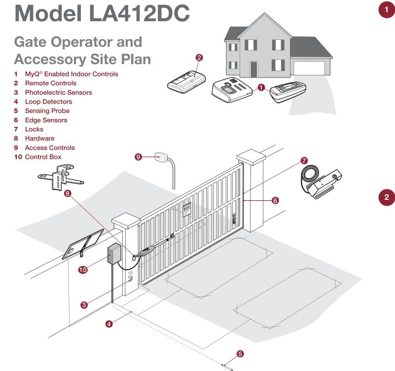
LiftMaster gate operators comply with UL 325 standards. Important: To be compliant with UL 325 and industry safety guidelines, qualified monitored external entrapment protection devices such as photoelectric sensors or edge sensors are required to be installed with this operator.
